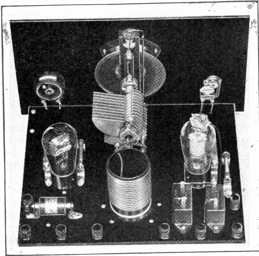
FIG. 5 REAR VIEW OF THE SHORT-WAVE RECEIVER ALONE. TO THIS WAS ADDED THE AUDIO CHANNEL TO FEED THE KINO LAMP.
